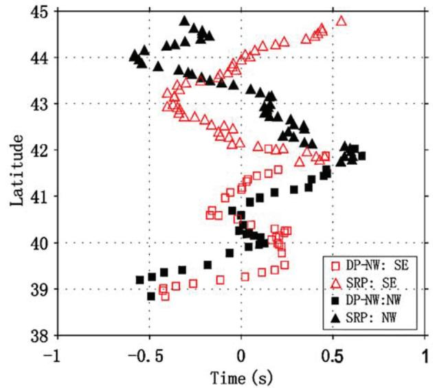
**Figure 2.** Teleseismic P-wave summary-ray residuals for the Deep Probe-Snake River Plain (DP-SRP) transect. Negative and positive residuals are late and early arrivals, respectively. Note that where the two arrays meet at 41.9°, the residuals from both back-azimuths are consistent, implying that any possible baseline shift between the two different relative residual data sets is insignificant.
