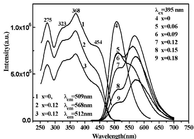
**Figure 3.** The excitation and emission spectra of  $\text{Ca}_3(\text{SiO}_4)\text{Cl}_2:0.09\text{Eu}^{2+},x\text{Mn}^{2+}$  ( $x = 0, 0.06, 0.09, 0.12, 0.15, 0.18$ ).
