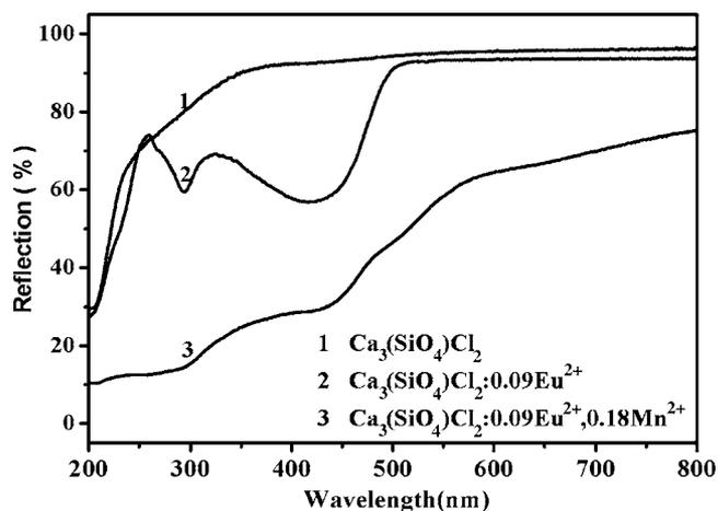
**Figure 2.** Powder diffuse reflection spectra of  $\text{Ca}_3(\text{SiO}_4)\text{Cl}_2$ ,  $\text{Ca}_3(\text{SiO}_4)\text{Cl}_2:0.09\text{Eu}^{2+}$ , and  $\text{Ca}_3(\text{SiO}_4)\text{Cl}_2:0.09\text{Eu}^{2+},0.18\text{Mn}^{2+}$ .
