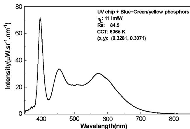
**Figure 13.** The electroluminescence spectra of the white LEDs based on UV chips, the blend of blue chlorophosphate and green/yellow  $\text{Ca}_3\text{SiO}_4\text{Cl}_2:\text{Eu}^{2+}, \text{Mn}^{2+}$  phosphors.
