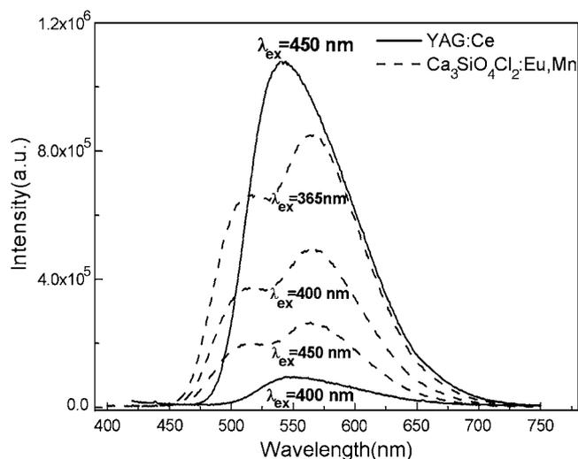
**Figure 11.** Comparison of the emission spectra of  $\text{Ca}_3(\text{SiO}_4)\text{Cl}_2:0.09\text{Eu}^{2+}, 0.12\text{Mn}^{2+}$  and YAG:Ce.
