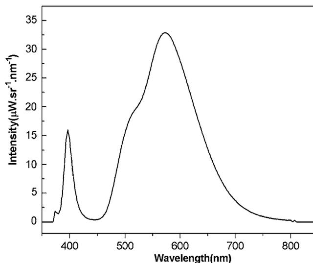
**Figure 12.** The electroluminescence spectra of the yellow LED based on  $\text{Ca}_3\text{SiO}_4\text{Cl}_2:\text{Eu}^{2+}, \text{Mn}^{2+}$  under  $I_F = 20$  mA.
