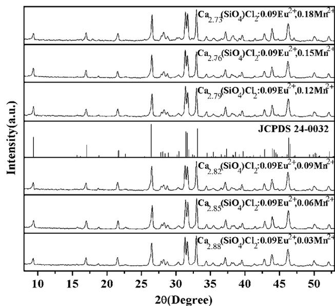
**Figure 1.** Powder XRD patterns of  $\text{Ca}_3(\text{SiO}_4)\text{Cl}_2$  (JCPDS 24-0032) and  $\text{Ca}_3(\text{SiO}_4)\text{Cl}_2:0.09\text{Eu}^{2+},x\text{Mn}^{2+}$  ( $x = 0.03, 0.06, 0.09, 0.12, 0.15, 0.18$ ).
