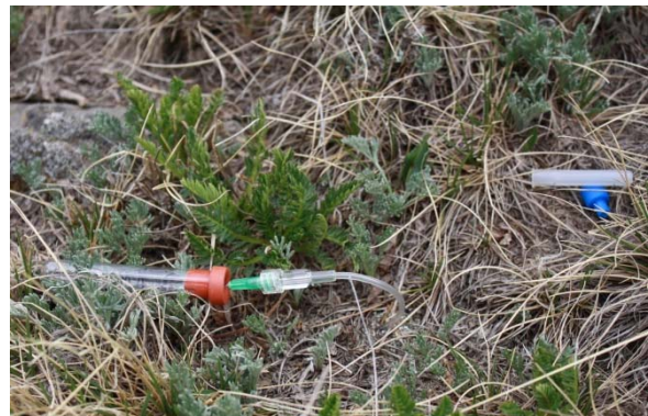
Figure 3. Soil lysimeter and attached vacutainer collecting soil water for analysis of mobile N (nitrate).
