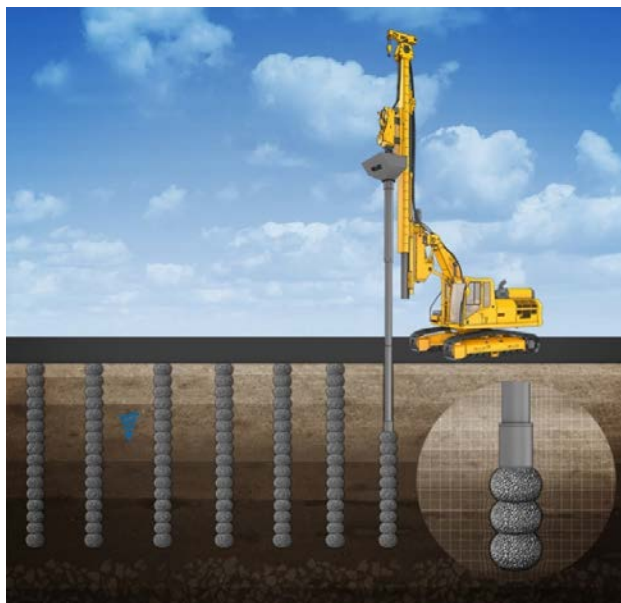
Figure 1. Engineered Aggregate Piers. Source: https://smediacacheak0.pinimg.com/736x/a9/30/10/a93010d5a9a9f473ac9a77ed4c585139.jpg
