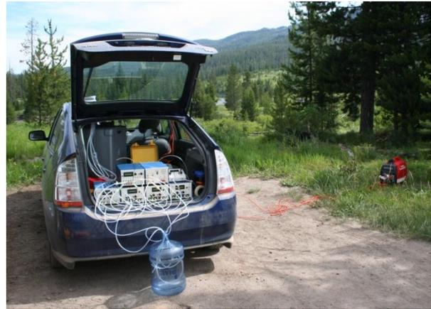
Figure 1. The metabolic chamber is powered through a portable generator (right) and all metabolic equipment is contained within the vehicle.
